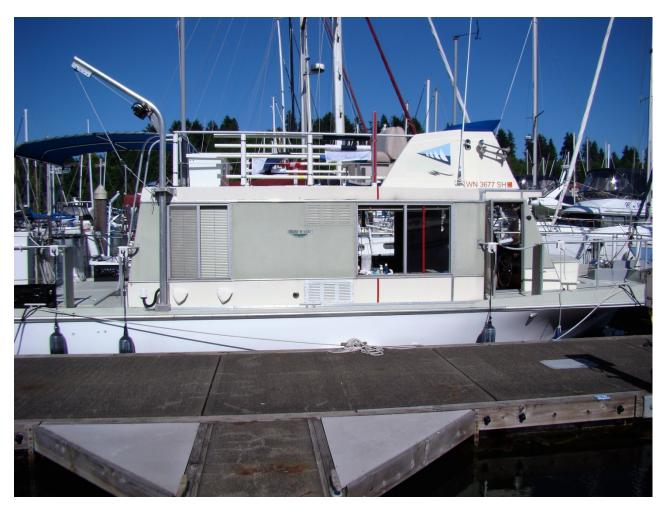
Starboard side: note the red stripe that denotes the start/finish line (when the sliding window is closed) During wet cold conditions boats can be finished from within the cabin by sighting through the red lines to the finish line mark. Note also the boom with winch for retrieving anyone who is in the water and needs to be lifted out with the aid of the Life Sling.
