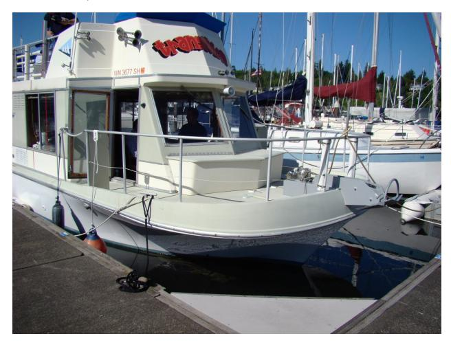
From the bow. Notice the upper deck, and of course the massive anchor roller and windlass on the bow. This makes it easy to set and adjust the start and finish lines without straining anyone's back. The anchor can be raised and lowered completely from inside the cabin without anyone having to go out on the deck. Horns mounted on the fly bridge are extremely loud and easy to hear over the flogging of sails and confusion as boats jockey for position prior to a race start.
