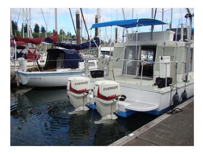
From the stern. Two 135 HP Evinrude outboard motors provide plenty of power and speed plus easy maneuvering to set marks. Note also the sturdy swim step/ engine mount. This was all part of the inboard engine replacement project that was an expensive surprise, but needed to be done. The original engines just up and died after the boat was placed into service. A lot of people would have given up at this point, but not Bill and Vicky.
